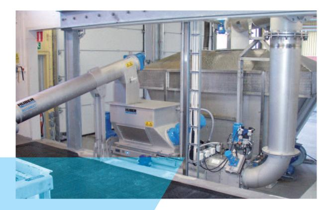
Screenings Wash Press for washout of organics and controlled high-pressure dewatering
