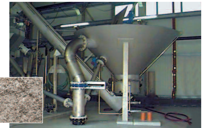
Washed grit from COANDA Grit Washer with < 3% loss on ignition, particle size up to 10 mm, DR > 90%
